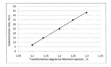
Fig. 1. Sedimentation rate (mL/s) versus PAA transformation degree by Mannich reaction (%)
