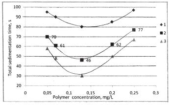
Fig. 2. Total sedimentation time versus polymer concentration (flocculation agent): 1-PAH; 2-PAM; 3-PAH+aluminium sulphate (40 mg/L)
